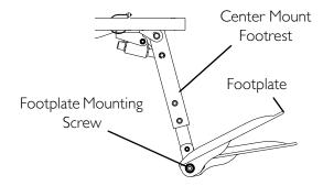
FIGURE 6.19 Adjusting the Footplate Angle - Before 2/15/07
